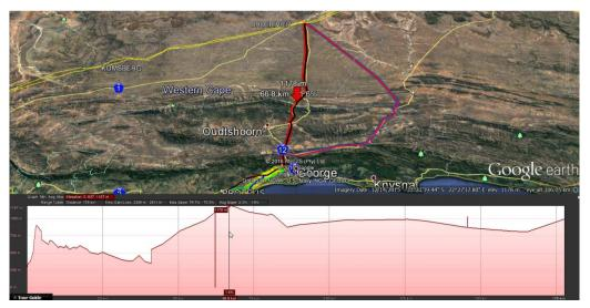
Figure 3: Elevation Profile for route alternative 1
